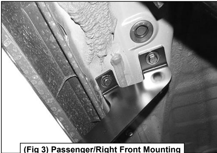
(Fig 3) Passenger/Right Front Mounting Bracket attached to the front location
