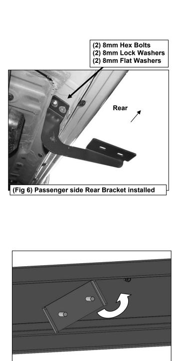
(Fig 8) Slide 8mm Double Bolt Plate into channel on bottom of Running Board
