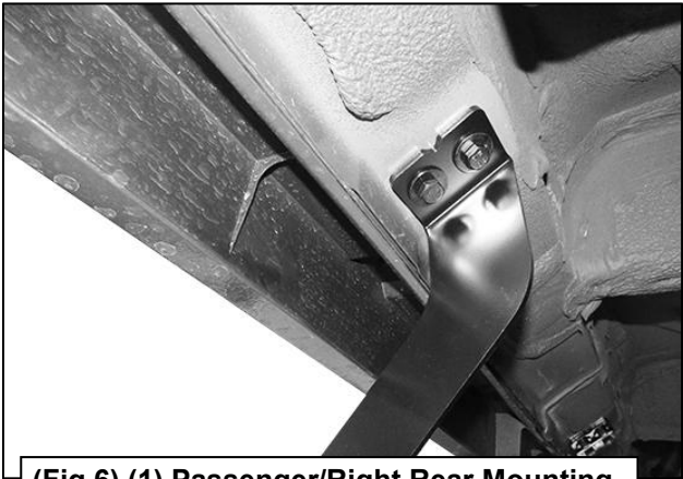
(Fig 6) (1) Passenger/Right Rear Mounting Bracket attached to the 2nd location
