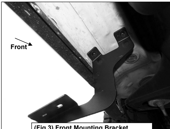
(Fig 3) Front Mounting Bracket attached to the front location
