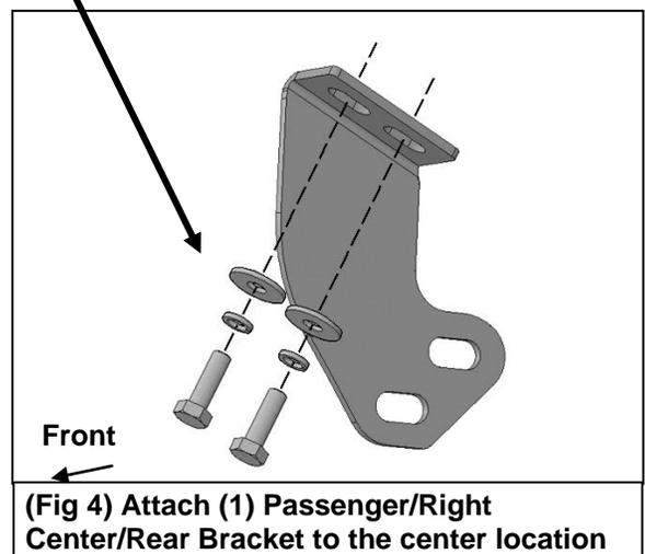
(Fig 4) Attach (1) Passenger/Right Center/Rear Bracket to the center location
