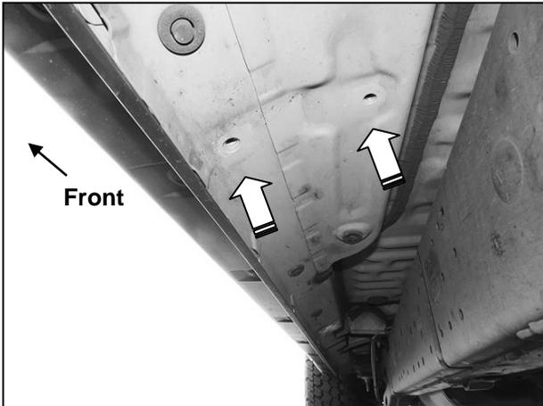
(Fig 1) Remove the plastic plugs (if equipped) or hex bolts from the threaded mounting holes in the floor panel. Passenger/right front mounting location pictured (arrows)
