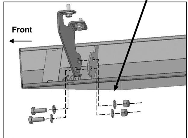
(Fig 6) Attach the Running Board to the back of the front Mounting Bracket
