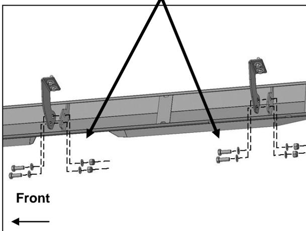
(Fig 7) Attach the Running Board to the back of the center and rear Mounting Brackets
