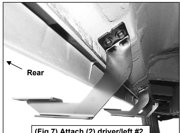
(Fig 7) Attach (2) driver/left #2, #3 and Rear Brackets to the #3 and rear mounting locations
