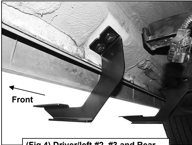
(Fig 4) Driver/left #2, #3 and Rear Bracket attached to the #2 location
