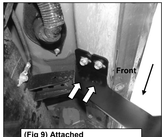
(Fig 7) Remove Plastic Plugs and attach Passenger/Right Rear bracket at rear mounting location
