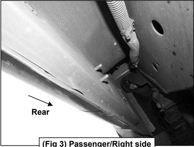
(Fig 3) Passenger/Right side rear mounting location
