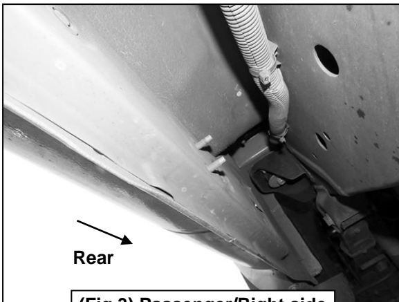
(Fig 3) Passenger/Right side rear mounting location
