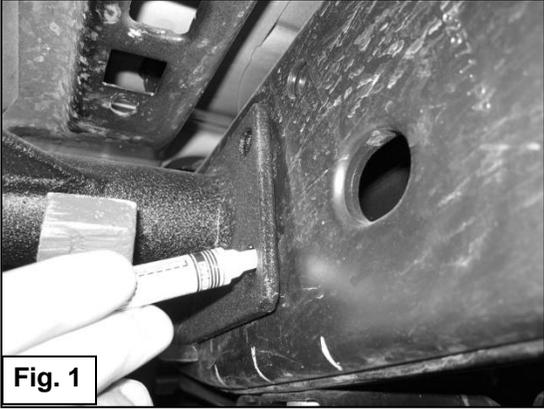
Hold the Running Board up to the side of the frame and level to the body. Mark the mounting holes onto the side of the frame
