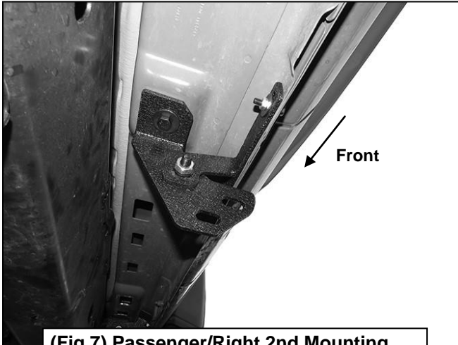
(Fig 7) Passenger/Right 2nd Mounting Bracket and (1) Center Support Bracket attached to the 2nd location
