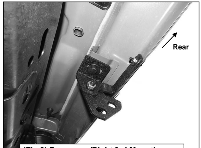
(Fig 8) Passenger/Right 3rd Mounting Bracket and (1) Center Support Bracket attached to the 3rd location
