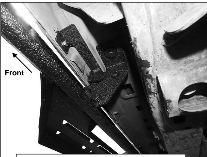
(Fig 11) Passenger/Right Running Board attached to the Front Mounting Bracket
