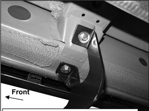
**(Fig 6) Center bracket-passenger side**
