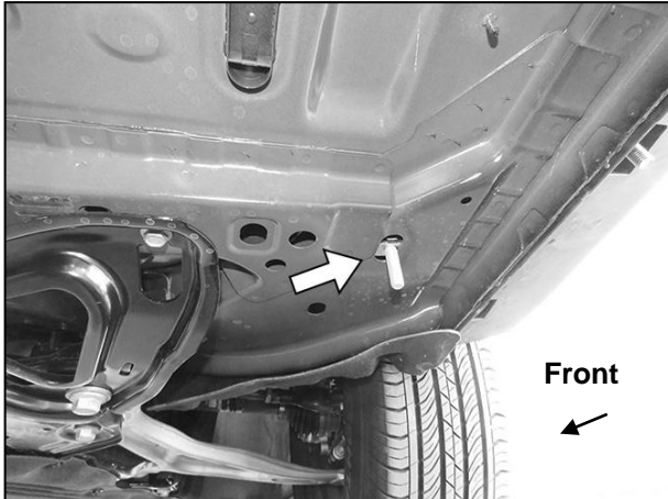
(Fig 15) Insert "Long" Bolt Plate into oval hole in front floor location (arrow)
