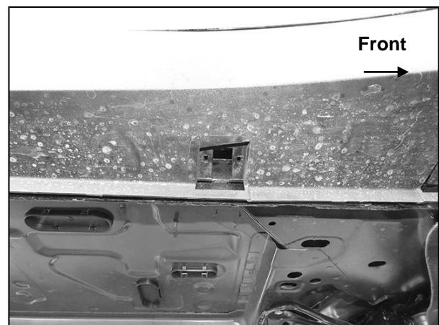
(Fig 2) Passenger/right #2 clip removed
