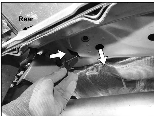
(Fig 19) Insert "Short" Bolt Plate into square hole and down through floor (arrow)
