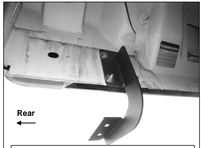
(Fig 8) Driver/left side rear Bracket installed
