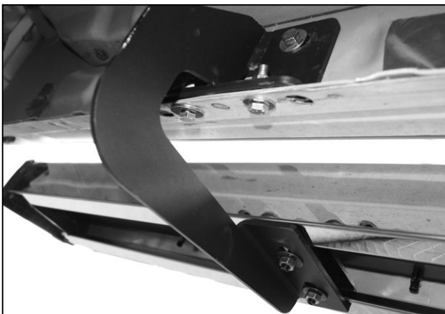
(Fig 12) Driver/left rear complete installation
