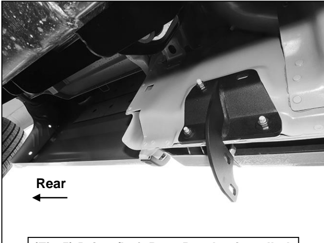
(Fig 5) Driver/Left Rear Bracket installed
