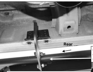
(Fig 10) Driver/left side Running Board attached to rear Bracket
