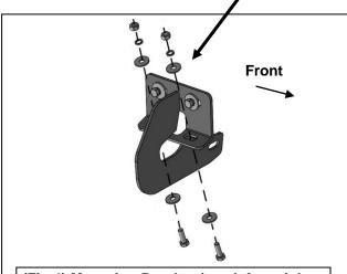
(Fig 4) Mounting Bracket (use left or right side) attached to pinch weld
