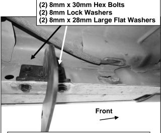
(Fig 5) Driver/left front Bracket installed
