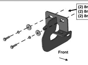
(Fig 3) Mounting Bracket (use left or right side) attached to inner body panel
