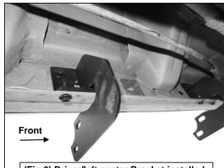
(Fig 6) Driver/left center Bracket installed
