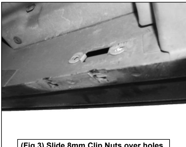
(Fig 3) Slide 8mm Clip Nuts over holes
