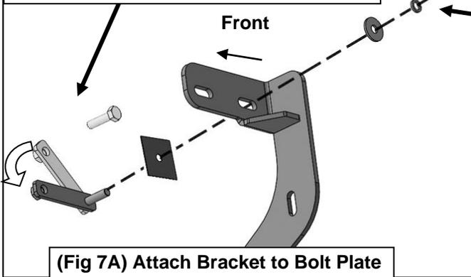
**(Fig 7A) Attach Bracket to Bolt Plate**
