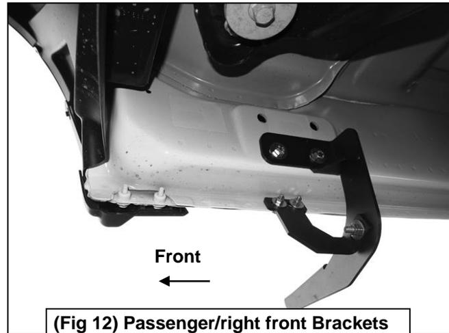
(Fig 12) Passenger/right front Brackets attached to body panel and pinch weld
