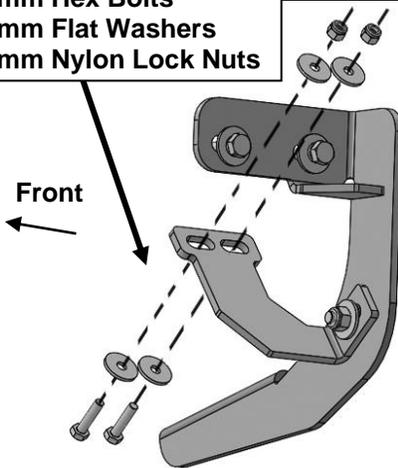
**IMPORTANT:** 2009-2012 models without holes in pinch weld will require drilling 1/4" holes through pinch weld to attach Support Brackets. Do complete installation of Running Boards first and level Running Boards before drilling holes for Support Brackets.
