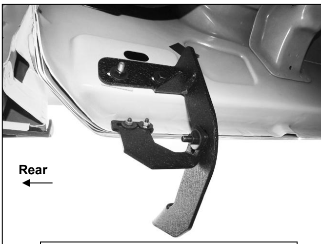
(Fig 16) Driver/left rear Brackets attached to body panel and pinch weld
