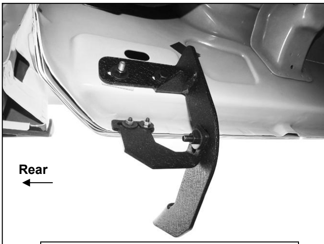
(Fig 16) Driver/left rear Brackets attached to body panel and pinch weld
