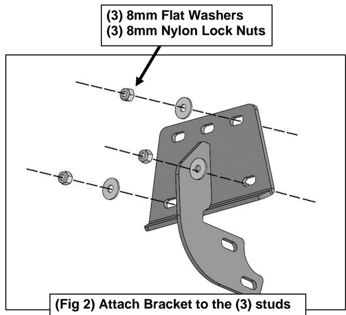
**(Fig 2) Attach Bracket to the (3) studs**
