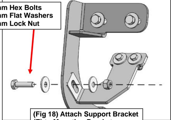
**(Fig 18) Attach Support Bracket (E) to Mounting Bracket**
