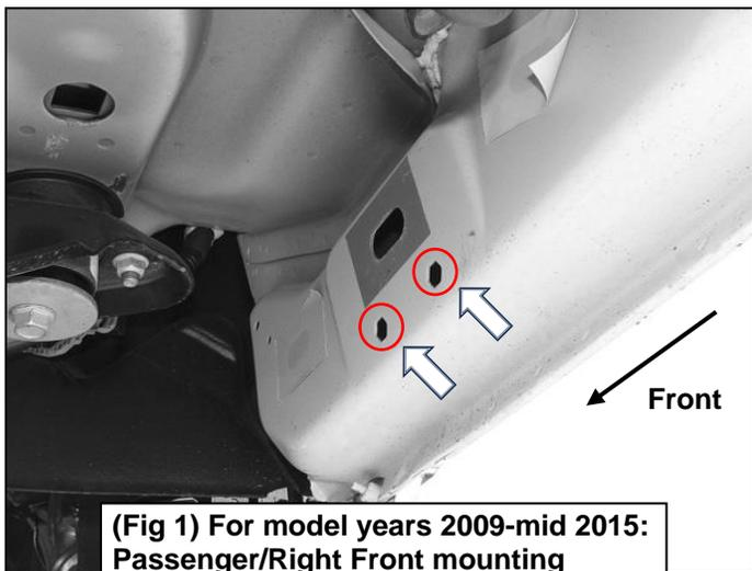
**(Fig 1) For model years 2009-mid 2015: Passenger/Right Front mounting location with hexagonal holes**
