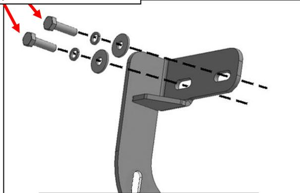
**(Fig 17b) Attach Passenger/Right Center Mounting Bracket directly to threaded holes**
