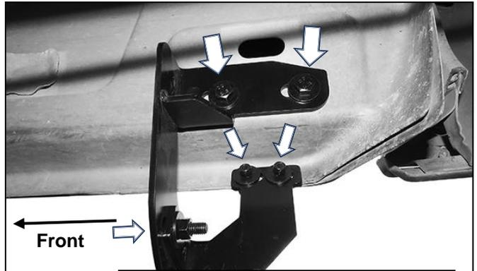
**(Fig 20) Attached Mounting Bracket with attached Support Bracket**
