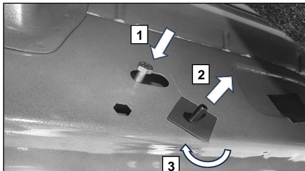
**(Fig 3) 1. Use the loose Hex Bolt as a handle. Insert the Bolt Plate into the oval hole
