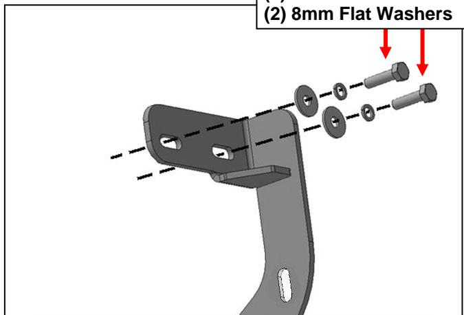
**(Fig 7) Attach Passenger/Right Front Mounting Bracket directly to threaded holes**
