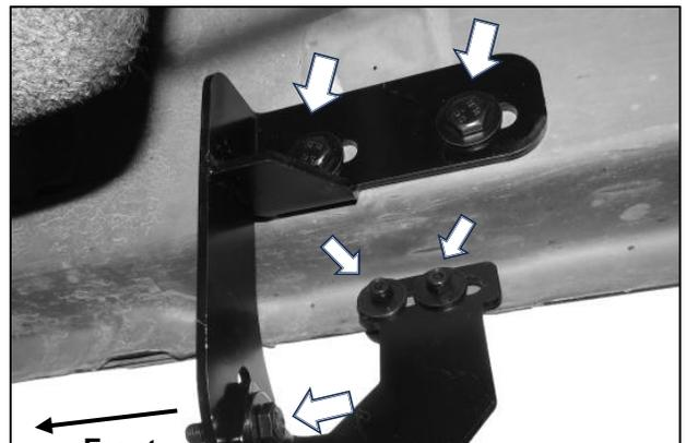
**(Fig 15) Attached Mounting Bracket with attached Support Bracket**
