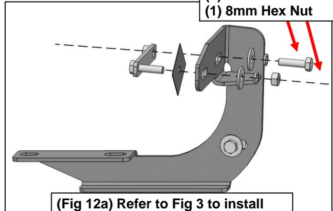
**(Fig 12a) Refer to Fig 3 to install Bolt Plates. Remove loose Hex Bolt and rotate Bolt Plate to line up nut with body panel and Mounting**
