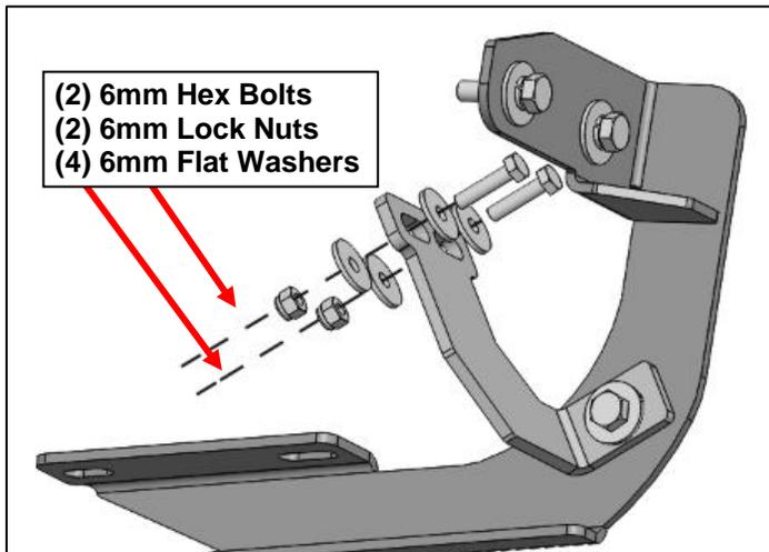
**(Fig 9) Attach Supporting Bracket to threaded holes in pinch weld**
