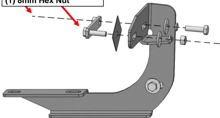
**(Fig 4) Remove loose Hex Bolt and rotate Bolt Plate to line up nut with body panel and Mounting Bracket then attach bracket to Bolt Plate**
