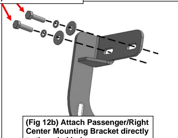
**(Fig 12b) Attach Passenger/Right Center Mounting Bracket directly to threaded holes**
