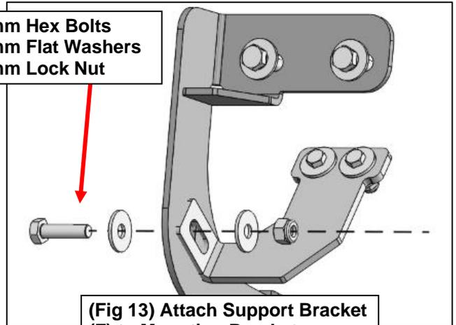
**(Fig 13) Attach Support Bracket (F) to Mounting Bracket**
