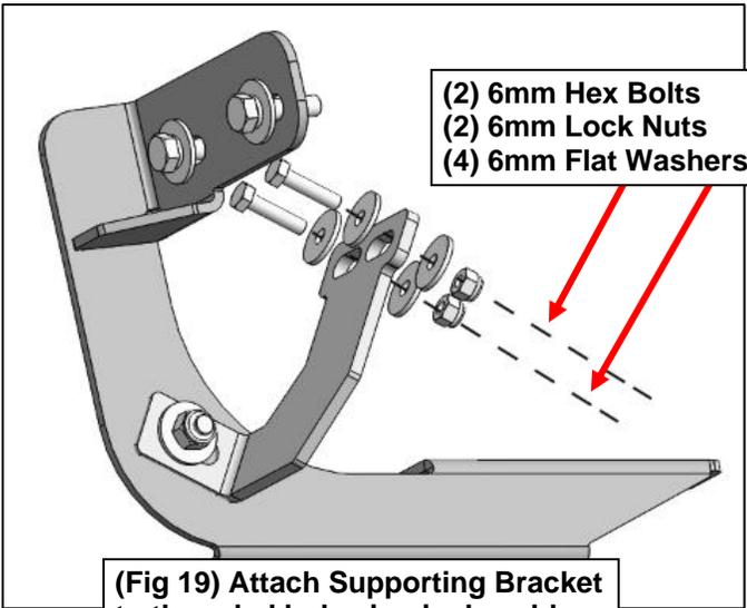
**(Fig 19) Attach Supporting Bracket to threaded holes in pinch weld**
