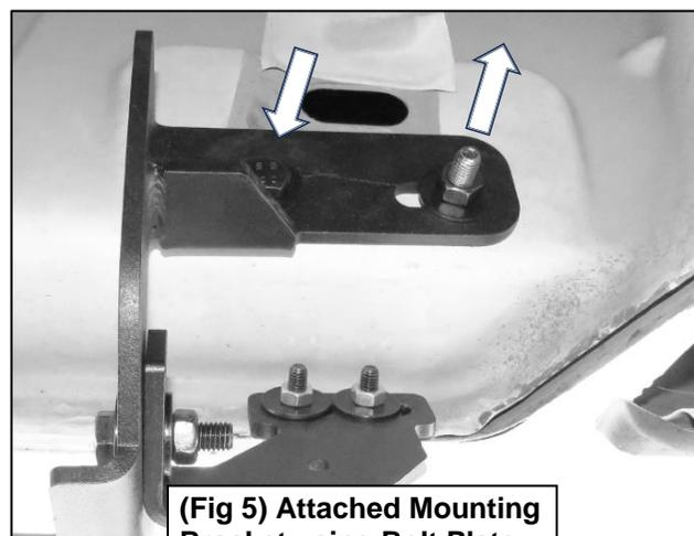
**(Fig 5) Attached Mounting Bracket using Bolt Plate**
