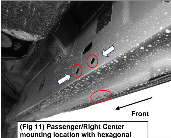
**(Fig 11) Passenger/Right Center mounting location with hexagonal holes. If hexagonal, refer to Fig 12a. If threaded, continue with Fig 12b**
