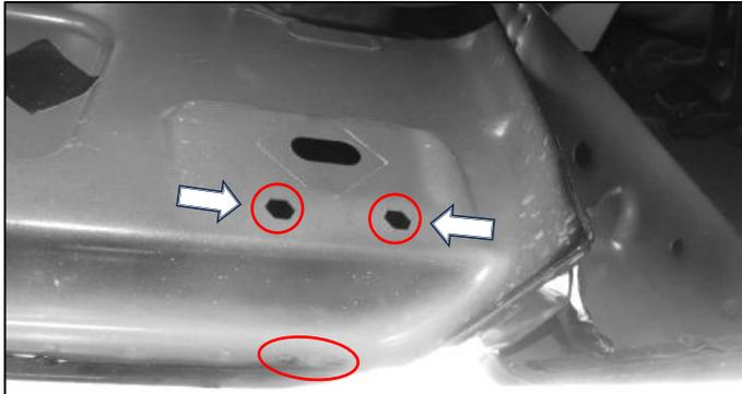
**(Fig 16) Passenger/Right Rear mounting location with hexagonal holes. If hexagonal, refer to Fig 17a. If threaded, continue with Fig 17b**
