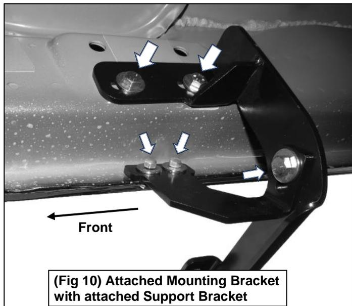
**(Fig 10) Attached Mounting Bracket with attached Support Bracket**
