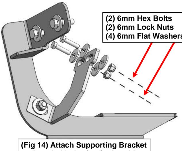
**(Fig 14) Attach Supporting Bracket to threaded holes in pinch weld**
