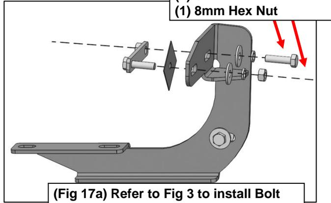
**(Fig 17a) Refer to Fig 3 to install Bolt Plates. Remove loose Hex Bolt and rotate Bolt Plate to line up nut with body panel and Mounting Bracket then attach bracket to Bolt Plate**
