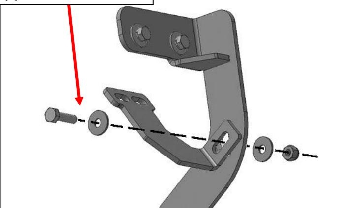
**(Fig 8) Attach Support Bracket (F) to Mounting Bracket**
