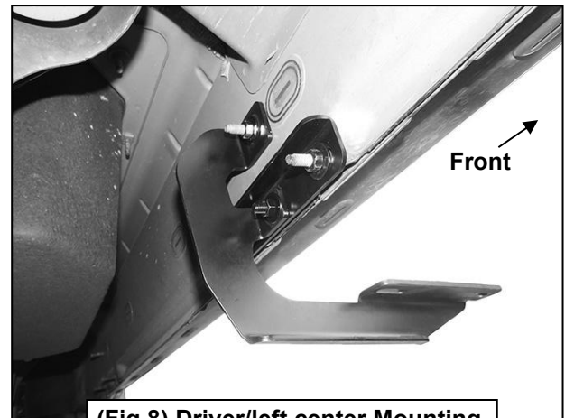
(Fig 8) Driver/left center Mounting Bracket assembly installed
