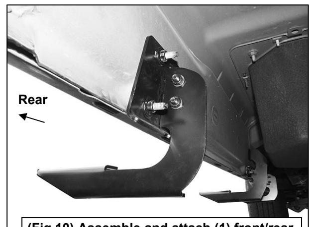
(Fig 10) Assemble and attach (1) front/rear Bracket Assembly to the rear mounting location (also see Figures 2 & 3)
