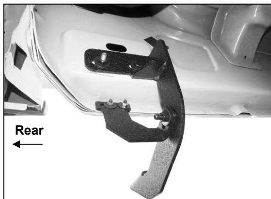
(Fig 15) Driver/left rear Brackets attached to body panel and pinch weld
