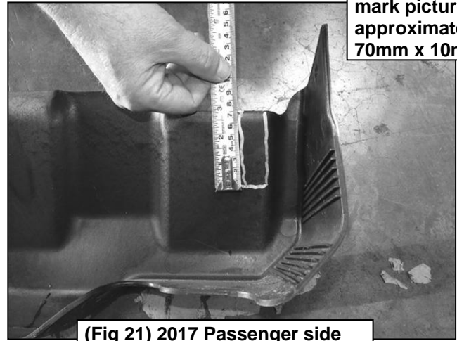
(Fig 21) 2017 Passenger side DEF cover marked for trimming
