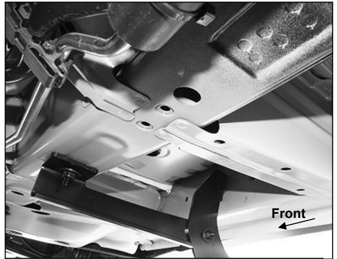
(Fig 7) Passenger/Right Front Brackets attached
