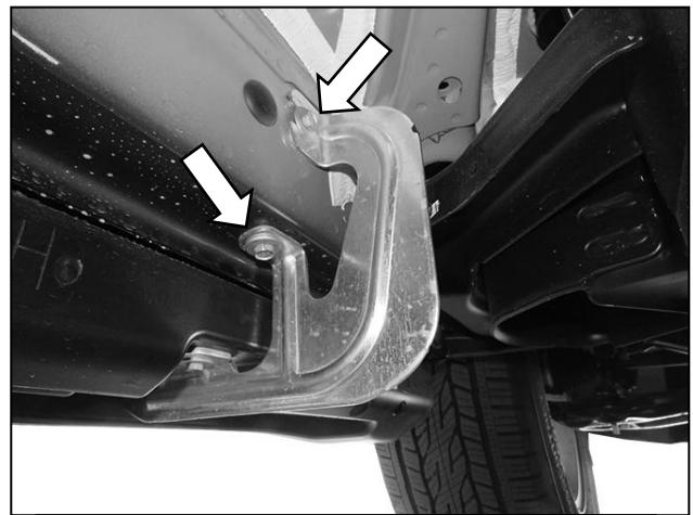
(Fig 2) Remove the bolts attaching the running board brackets to the rocker panel
