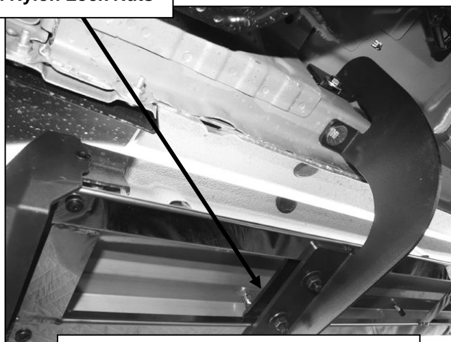
(Fig 12) Passenger side front Mounting Bracket attached to Running Board
