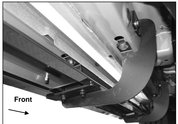
(Fig 10) Driver side Front and Center Mounting Brackets attached to Running Board
