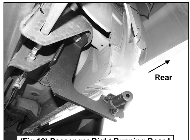
(Fig 19) Passenger Right Running Board attached to the Rear Mounting Bracket
