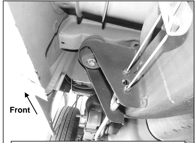
(Fig 13) Passenger/Right rear mounting location. Temporarily remove the body bolt
