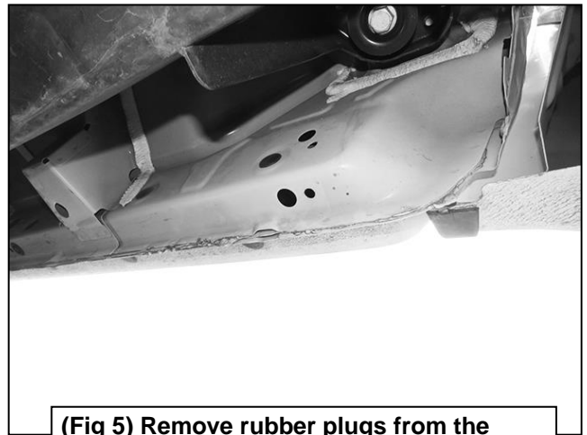
(Fig 5) Remove rubber plugs from the Passenger/Right rear mounting location
