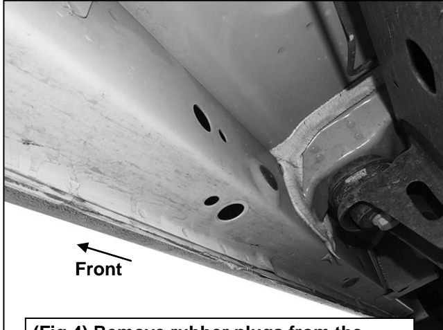
(Fig 4) Remove rubber plugs from the Passenger/Right center mounting location
