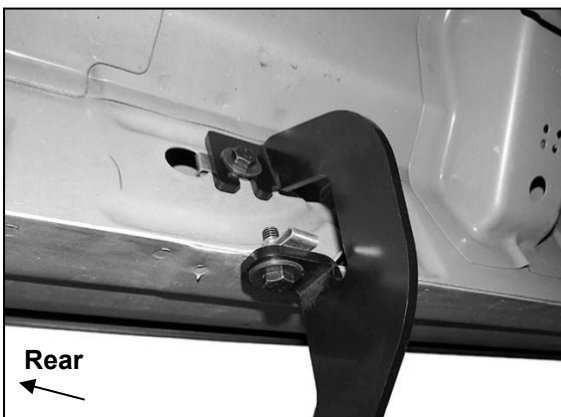
(Fig 8) Example of driver/left rear Bracket attached to location with 8mm Clip Nuts
