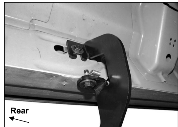
(Fig 7) Example of driver/left rear bracket attached to location with 8mm Clip Nuts
