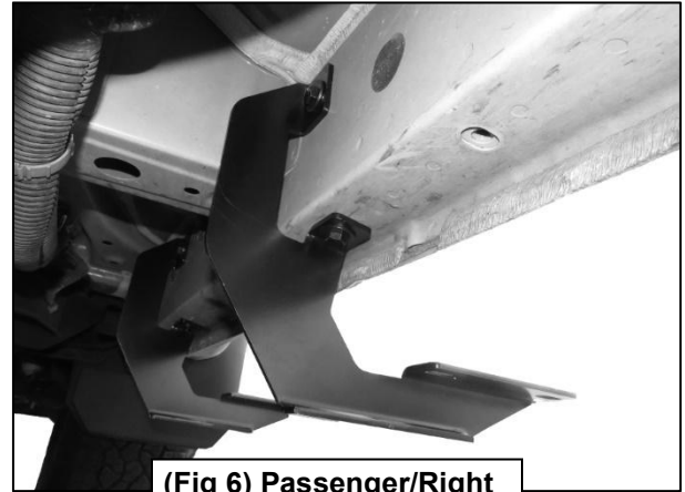
(Fig 6) Passenger/Right #2 Bracket installed
