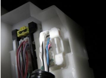
On the white connector, identify the Blue and White wires. Connect the High and Low wires from the main harness (J) using the supplied wire taps (L). After successfully connecting the wires, return the connector back into its place and check that it is secure.
