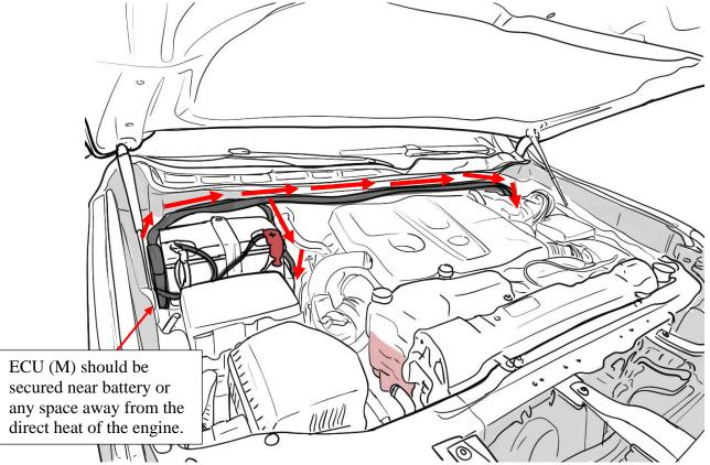
Route the shorter (marked "Passenger-side") leg of the harness down the Passenger-side wheel well. **Be sure to avoid contact with any moving or hot engine components.** Attach and secure the main harness (J) with supplied cable ties.
