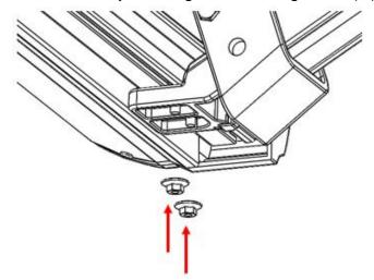
Once the board is adjusted, plug in main harness (J) connector to return power to the linkage arms. Open and close doors several times to deploy and retract the steps to settle the steps into their natural alignment. After cycling the step, tighten all hardware on the board and brackets.
