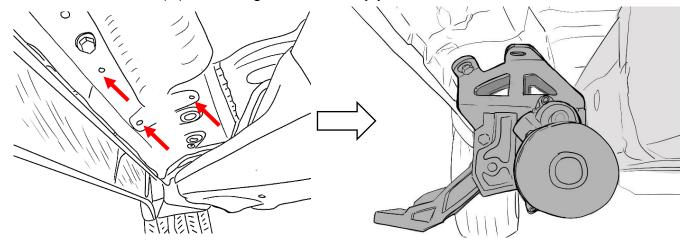
Locate rear mounting points. Next, line up rear mounting bracket slots to the threaded inserts and place Driver Side/Left Rear Bracket Assembly (B) onto rocker panel. Then fasten Hex Bolts (H), Lock Washers (I), and Flat washers (G). Do not tighten all the way yet.
