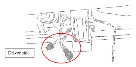
Plug in LED lights (N) into LED Y-Harness (K) and attach them to the bottom of the rocker panel. Use provided 3M double sided adhesive tape on back of LED light (N). Replace Fuse into Fuse Box.
