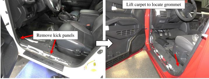
Locate the white OEM CAN Junction connector under the steering wheel, behind the kick panel. Be sure vehicle is not powered on. Slide the connector out of the holding junction by pushing the locking tab in the center and pulling downwards for easier access to wires.
