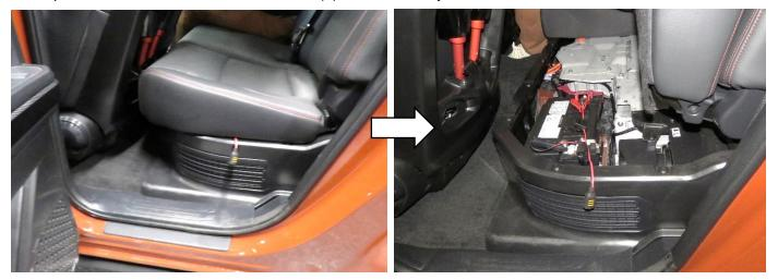
Route the main harness (J) around the battery and along the inside of the cabin. Find a good spot to hide the ECU. The Driver-side branch of the main harness must route down to the outside of the cabin to the Driver-side motor, on the underside. Connect the Short LED Y-harness too. **Be sure to avoid contact with the steering column and hot exhaust pipes.**
