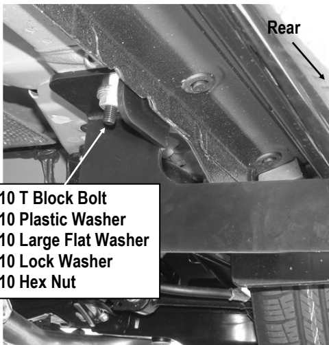
(Fig 9) Driver Side Rear Mounting Bracket Installation
