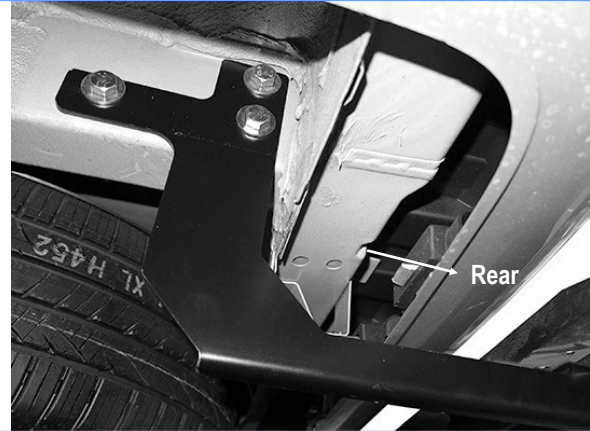
(Fig 3) Driver Side Mounting Bracket Installed
