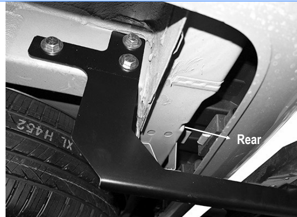
(Fig 3) Driver Side Mounting Bracket Installed
