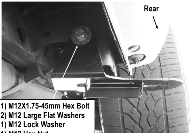
(Fig 7) Driver Rear Mounting Bracket Installed
