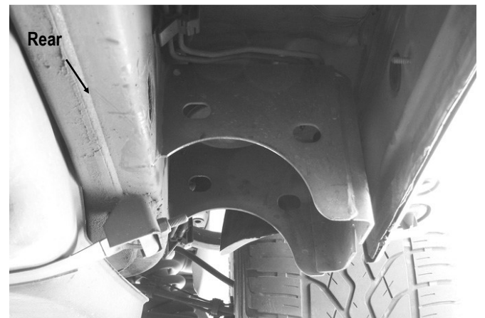
(Fig 5) Driver Side Rear Body Mount Location (After Plastic Cover Removed)
