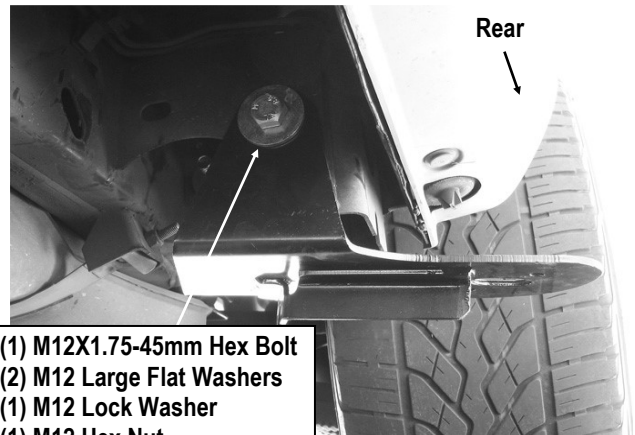
(Fig 7) Driver Rear Mounting Bracket Installed
