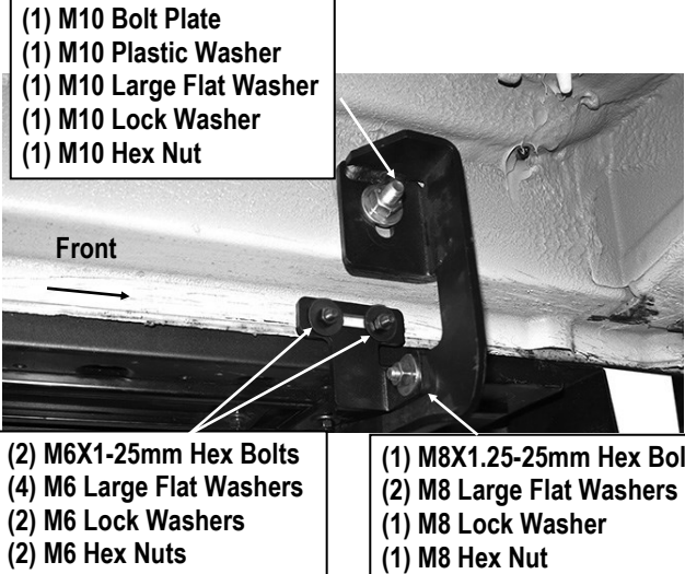
(Fig 16) Driver Side Front Bracket Installation
