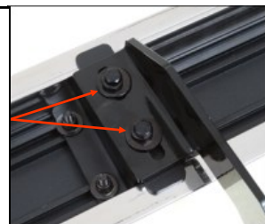
(Fig 11) Step Bar Installed on Bracket Installed (Example)
