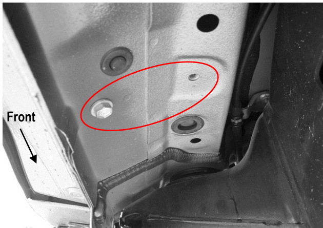
(Fig 1) Driver Side Front Mounting Location
