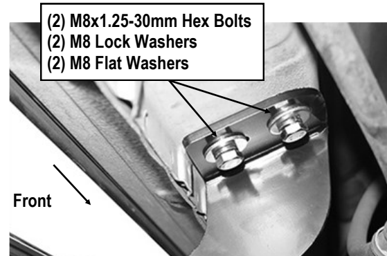
(Fig 4) Driver Center Mounting Bracket Installed
