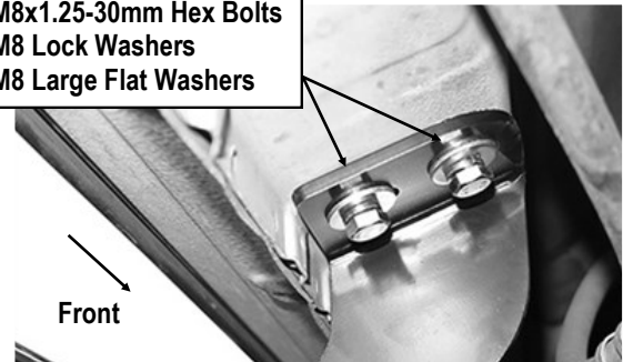
(Fig 7) Driver Center Mounting Bracket Installed
