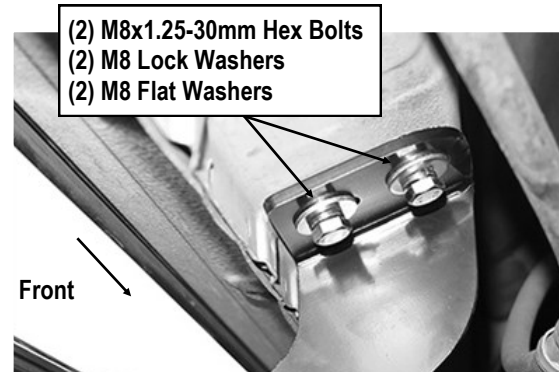
(Fig 4) Driver Center Mounting Bracket Installed
