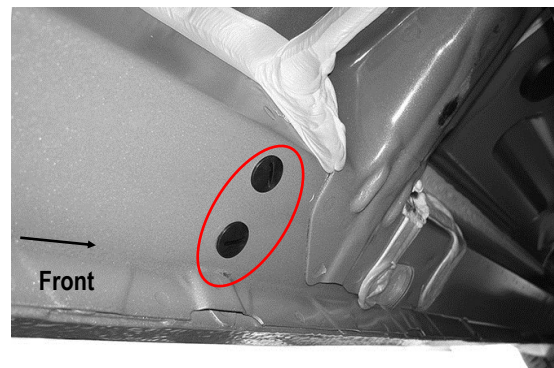
(Fig 3) Example of Driver Side Center & Rear Mounting Location
