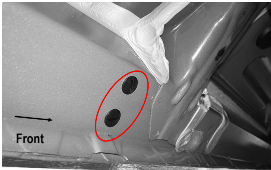
(Fig 3) Example Of Driver Side Center & Rear Mounting Location
