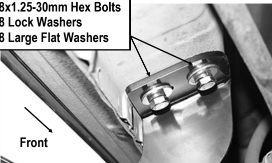
(Fig 4) Driver Center Mounting Bracket Installed
