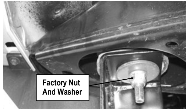
(Fig 2) Driver Rear Mounting Bracket Installation
